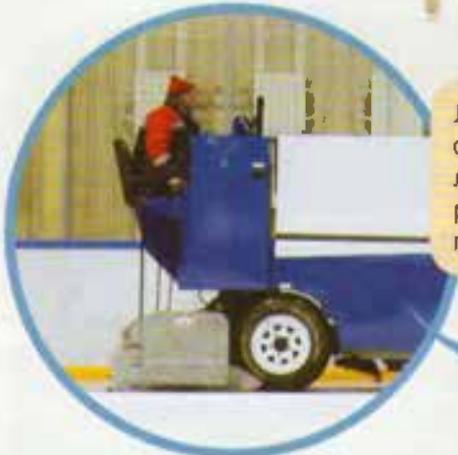
A circular inset image showing a person in a red jacket operating a blue ice resurfacing machine on an ice rink. The machine has a large wheel and a hopper for water.
